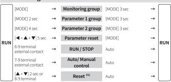
01) In the event of system anomalies and alarms, RESET input restarts the power controller. (parameters are not reset.)
