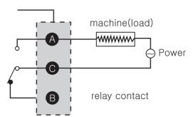
※ Relay contact capacity - less than 250VAC 2A In case of using the load exceeding the capacity of the contact, it caused fused contact, connection error.
