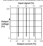
It outputs a constant current proportional to the control input so that the output current does not fluctuate against fluctuations in power voltage and load resistance fluctuations of loads (platinum, molybdenum, tungsten, etc.) in which the temperature coefficient of electrical resistance varies significantly from 6 to 12 times the normal temperature
