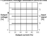
It outputs a constant voltage proportional to the control input so that the output voltage does not fluctuate against fluctuations upon in power voltage and load resistance fluctuation in power voltage and load resistance fluctuations of loads (iron, chromium, signal nichrome, etc.) with a small electrical [%] resistance temperature coefficients
